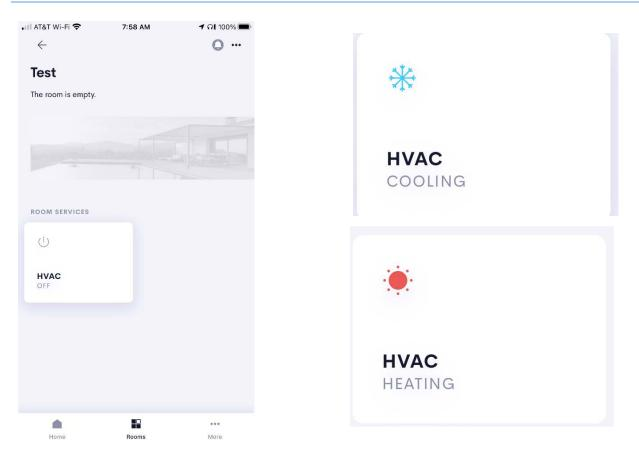
The above 3 images show the feedback as the HVAC system is switched from Off, to Cool, and then to Heat.
