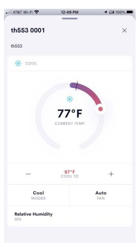
From this screen you can change the operating mode (off, cool, heat) and the fan mode (auto, on).
