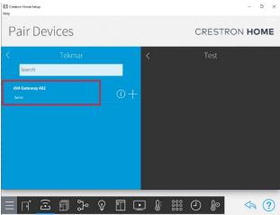
After selecting the "+" to add the extension you will be prompted to enter a unique name and select where the RS232 cable is connected (see below)
