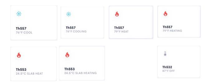
From left to right, top to bottom: Cool, Cooling, Heat, Heating, Slab Heat, Slab Heating, and Off.
