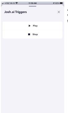
After touching the room/home screen tile, a list of available commands will be displayed. Simply touching the requested command will trigger the corresponding HTTP(s) Put.
