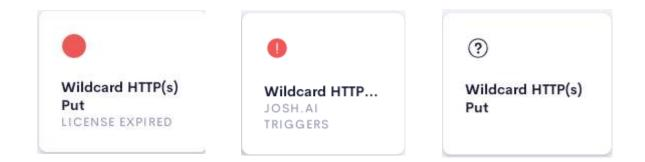
After 2 hours, without the proper license key having been installed, a license expired notice will be displayed as shown on the left image. The middle image indicates that there is an issue with the command string on one or more commands in the installer options. The right image indicates the extension has been correctly setup.
