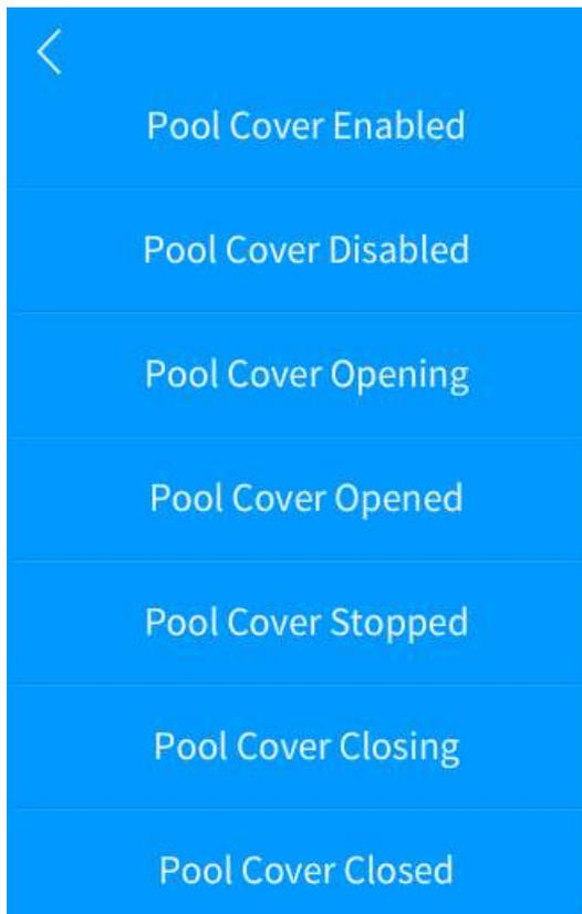
**Pool Cover Enabled** - enable normal extension functions.
