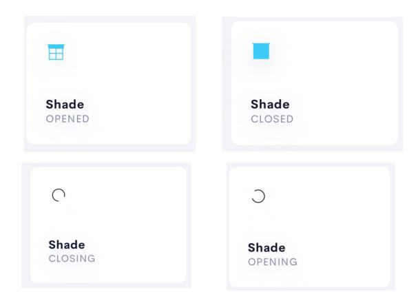
The above 4 images show the feedback as the shades goes from being opened, closed, opening, and closing. Opening and closing states will show a spinning circle for the number of seconds defined in the installer options.
