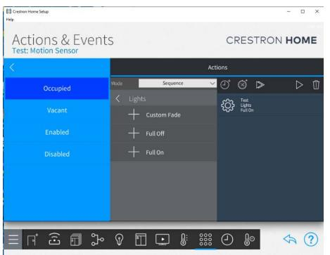
**Occupied** – Event that is executed when the Motion Buffer occupancy action has been triggered
